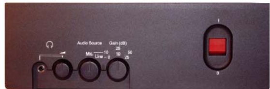
Ethernet Broadcast Unit (EBU) Controls AIM and streams audio over Ethernet
