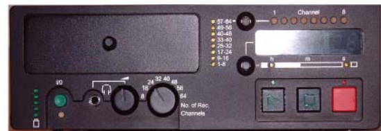
Hard Disk Recorder Receives streaming audio and stores on USB2 disk drive
